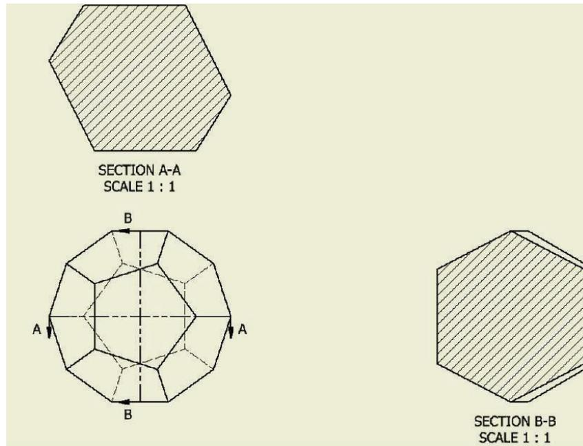
**Figure 5. Sectional View of Dodecahedron**
