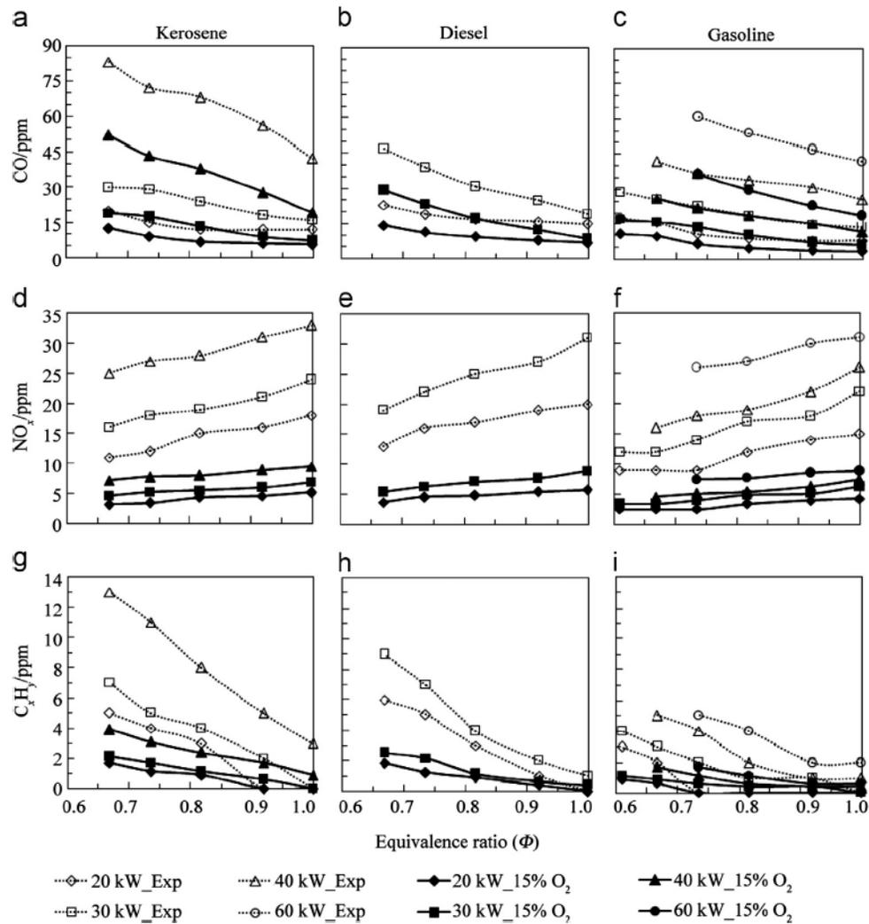
Figure 7: Pollutant emissions variation with equivalence ratio of different thermal inputs and three different fuels of kerosene, diesel and gasoline emissions.
