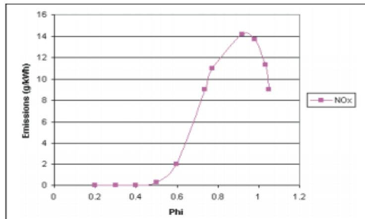
Figure 3-8 Emissions For A Hydrogen Engine
