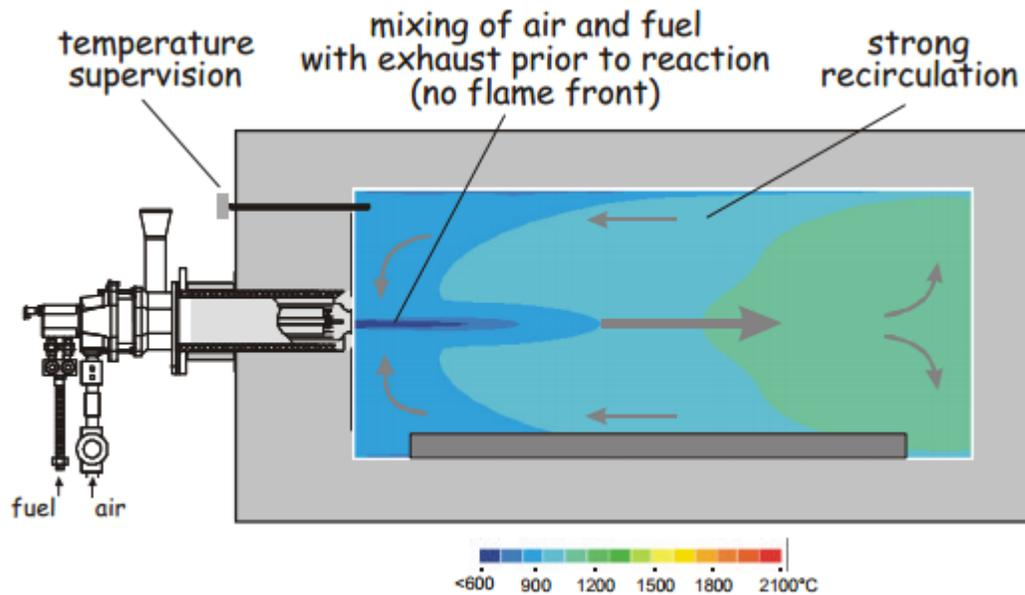
*Figure 6: Schematic diagram of flameless combustion*
