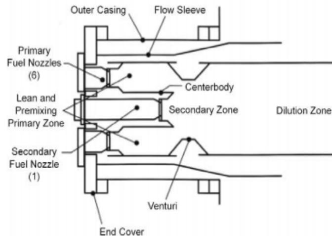
Figure 3: LPM combustion chamber
