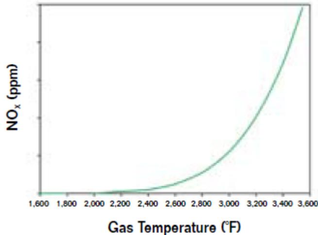
*Figure 1: NO<sub>x</sub> formation vs. temperature*
