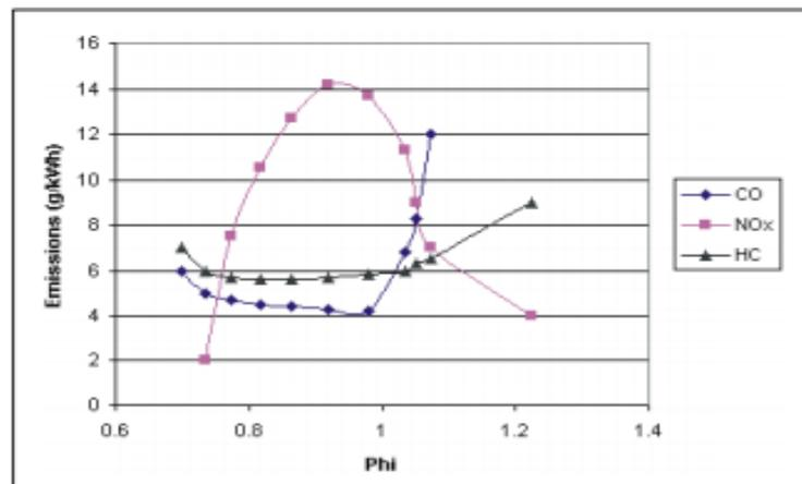
Figure 3-9 Emissions For A Gasoline Engine
