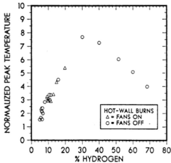
*Figure 8: Normalized peak Temperature vs. % hydrogen (Marshall, B. 1986)*
