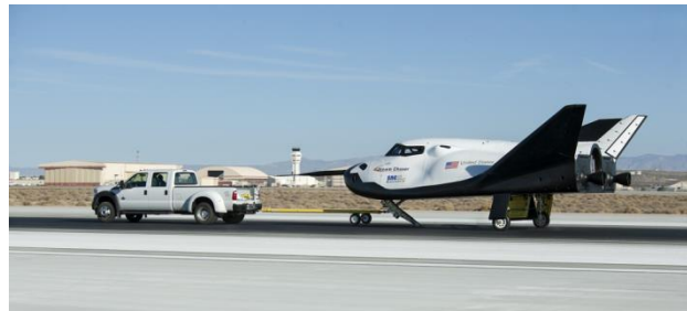
Figure 13. Dream Chaser Ground Tow Testing at Edwards Air Force Base. The Dream Chaser was tow-tested for more than 20 miles with no damage to the runways at Edwards Air Force Base, proving the compatibility of the skid with an existing runway.
