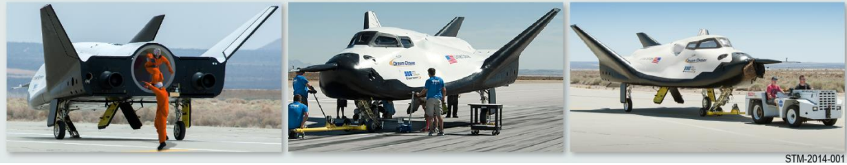
Figure 10. Dream Chaser Removal from Runway and Crew Egress. The Dream Chaser's design allows unassisted crew egress at any landing site without the need for special equipment. This operation nominally occurs after the vehicle has been towed off the runway. The minimum equipment needed to quickly remove the vehicle from the runway is enabled by the low toxicity and low hazard levels of the Dream Chaser design, thus minimizing the impact on day-to-day operations at a public-use landing site.
