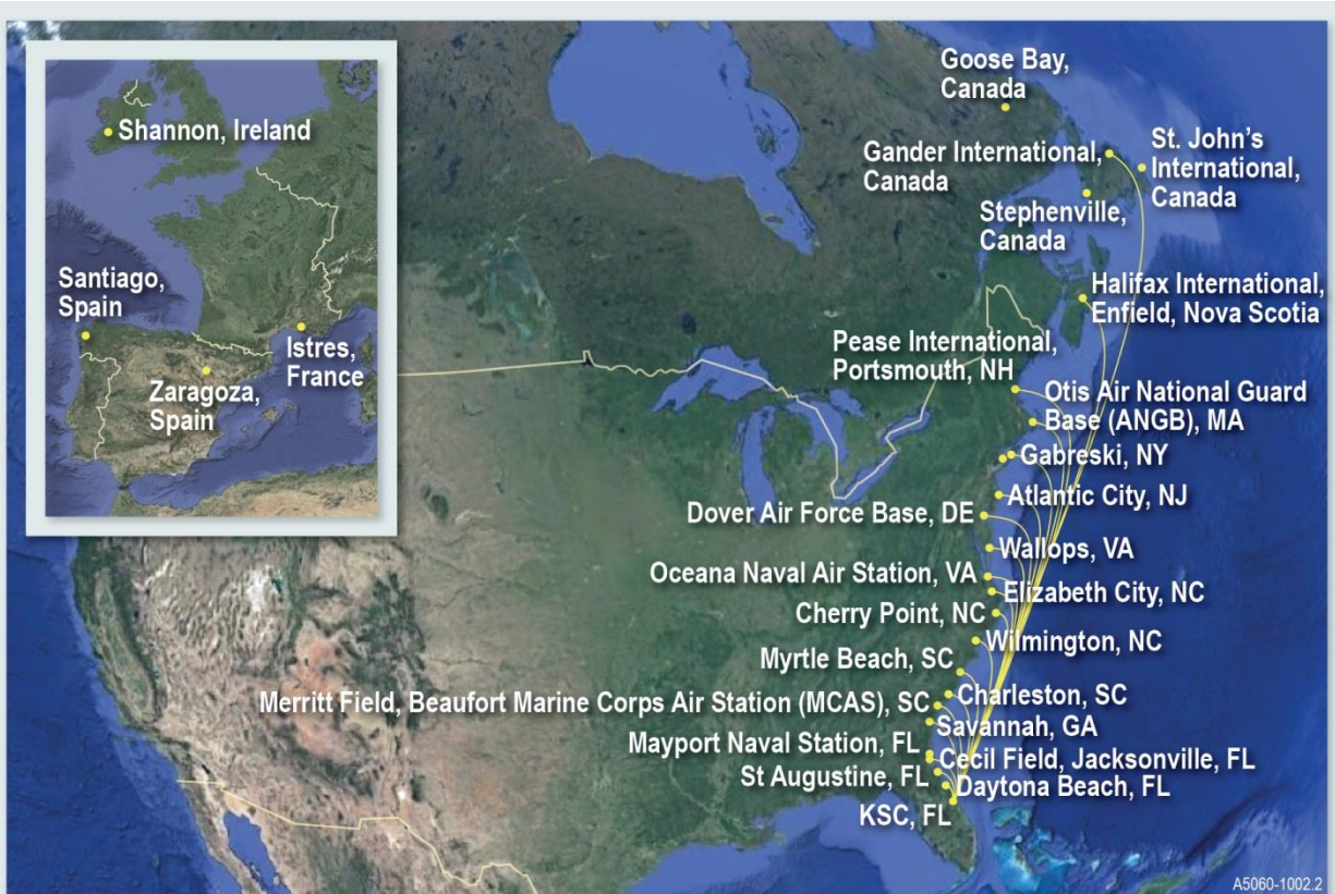
Figure 4. Abort Sites Along Ascent Flight Path. The Dream Chaser lifting body with a cross range of 1,100 nmi is capable of landing at any of the identified runways during ascent, thus representing a significant benefit for crew, payload, and vehicle safety.
