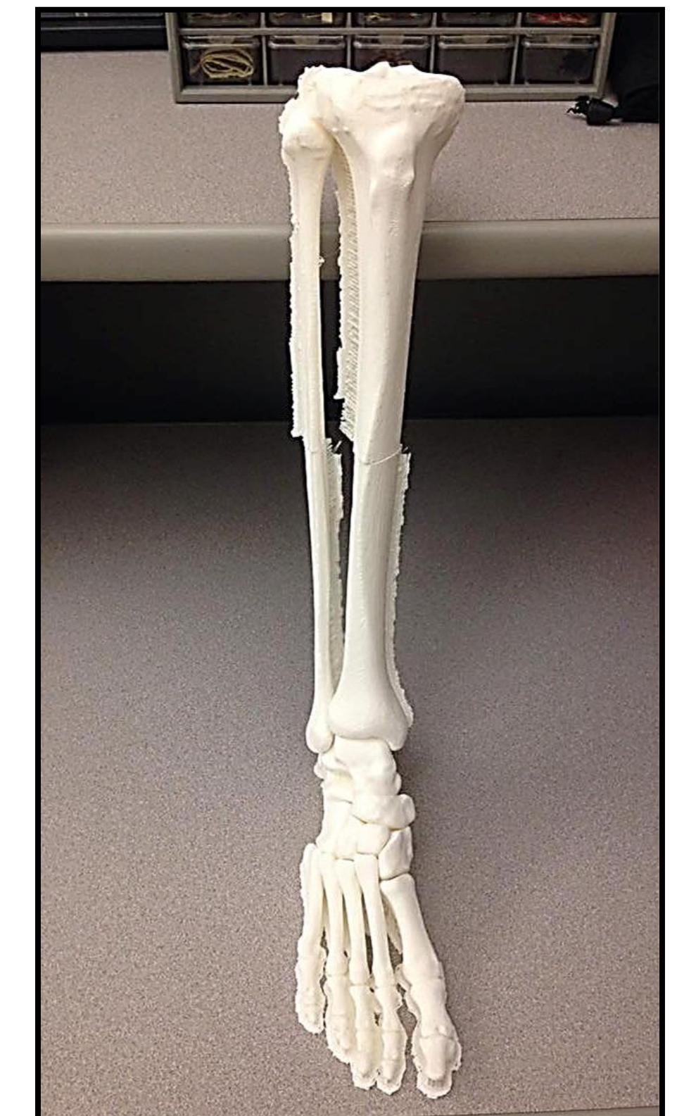
Figure 10. Foot and tibia have been 3D printed with a scaling factor of 4
