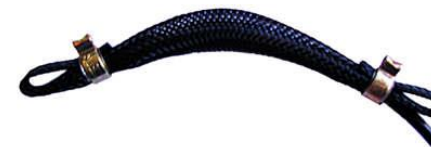
Figure 9. McKibben air muscles have been chosen to replicate the individual force vs. stretch curves. By varying the pressure, the passive muscle force can be adjusted
