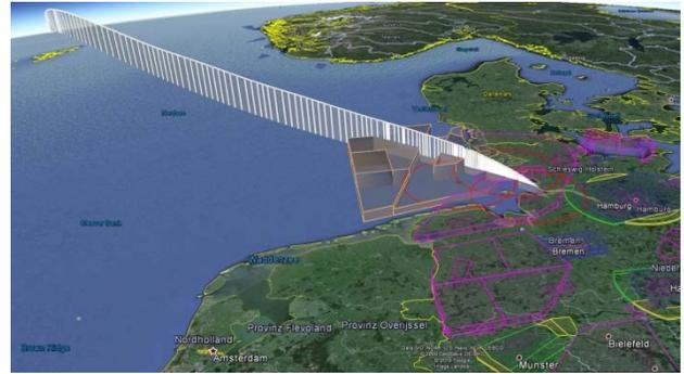
**Figure 2: SpaceLiner descent trajectory for destination in northern Germany; showing also danger areas, restricted areas and temporary restricted areas within German airspace<sup>1</sup>**
