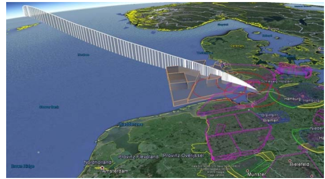
Figure 2: SpaceLiner descent trajectory for destination in northern Germany; showing also danger areas, restricted areas and temporary restricted areas within German airspace 1
