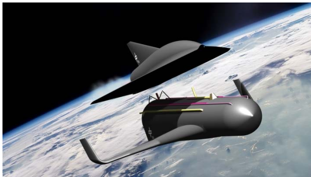
Figure 1: The SpaceLiner reusable booster and passenger stage during separation (DLR SART)
