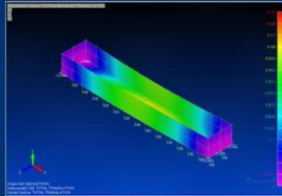
Nei Nastran is a finite element analysis solver used to generate approximate solutions for both nonlinear and linear stresses, dynamics, and heat transfer characteristics of a specified structure. Implementing differential equations and the associated structural boundary conditions this software segments the model into "N" number of finite elements and the individual analysis of these elements are combined to produce the a more accurate approximation for the structure in its entirety.
