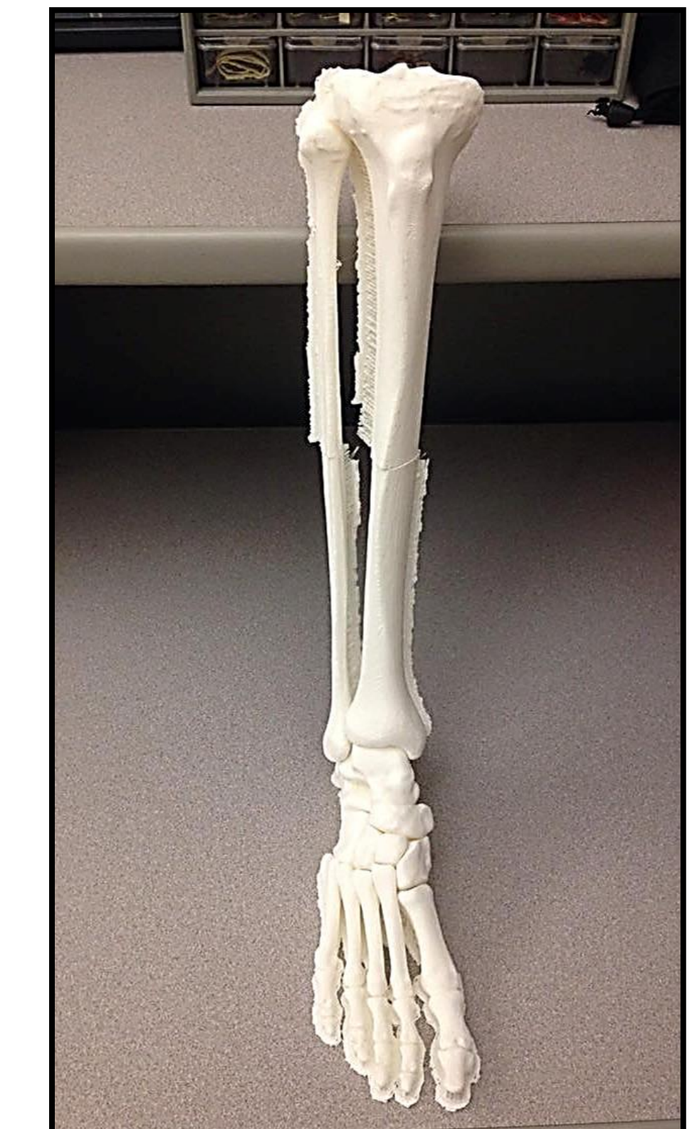
Figure 10. Foot and tibia have been printed with a scaling factor of 4
