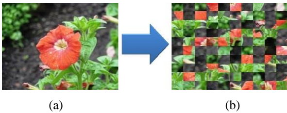
Figure 2 Frame Processing with the Proposed Sub-Frames Toral Automorphism Algorithm. (a) Original Frame with H \times W Dimensions, (b) Original Frame Divided and Processed with 10 \times 10 Subframes, N=10 , n=2 , and k=5 .
