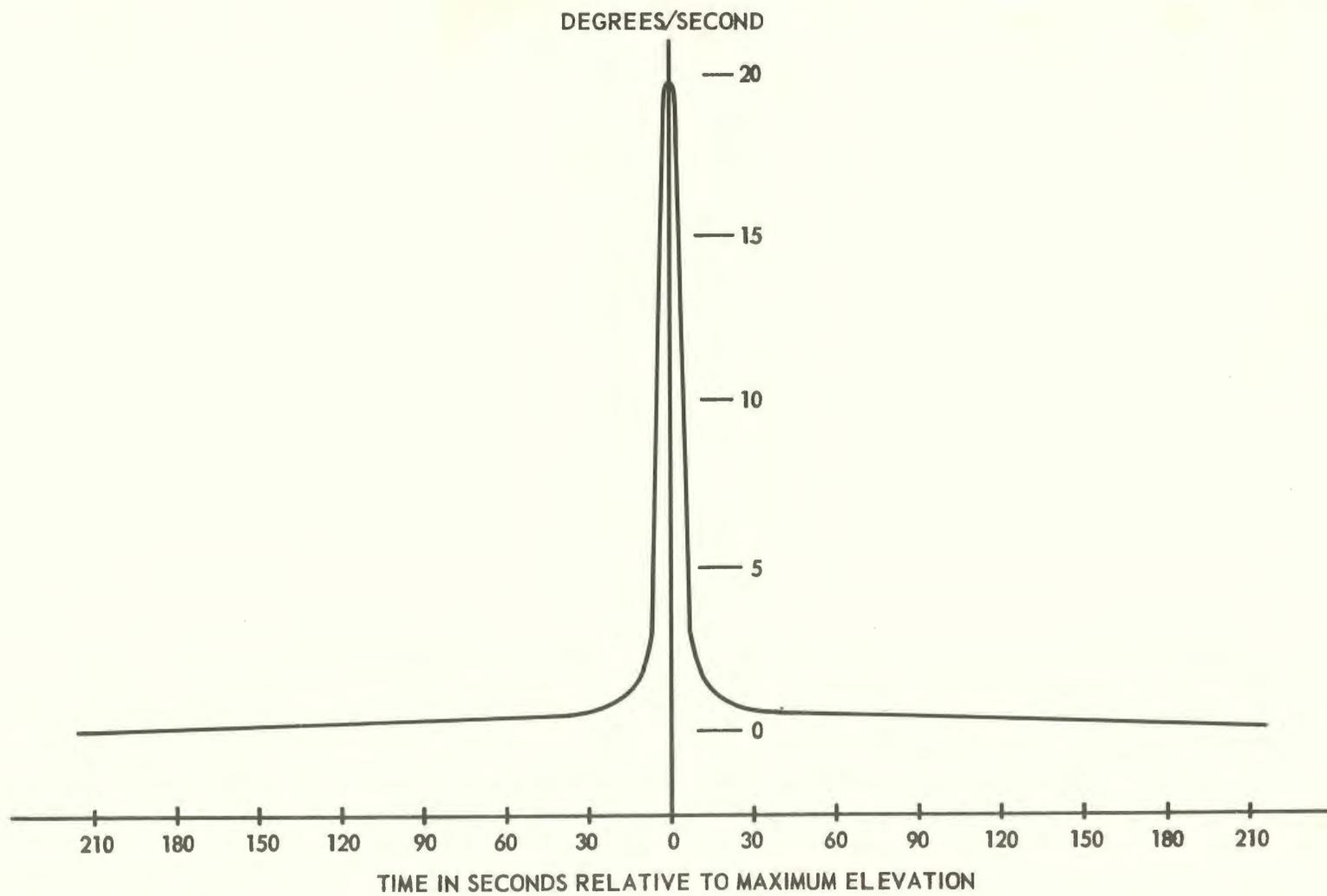
FIGURE 5 DOPPLER FREQUENCY SHIFT AND RATE FOR 100-NM CIRCULAR ORBIT WITH TRANSMITTER FREQUENCY OF 2300 MHZ
