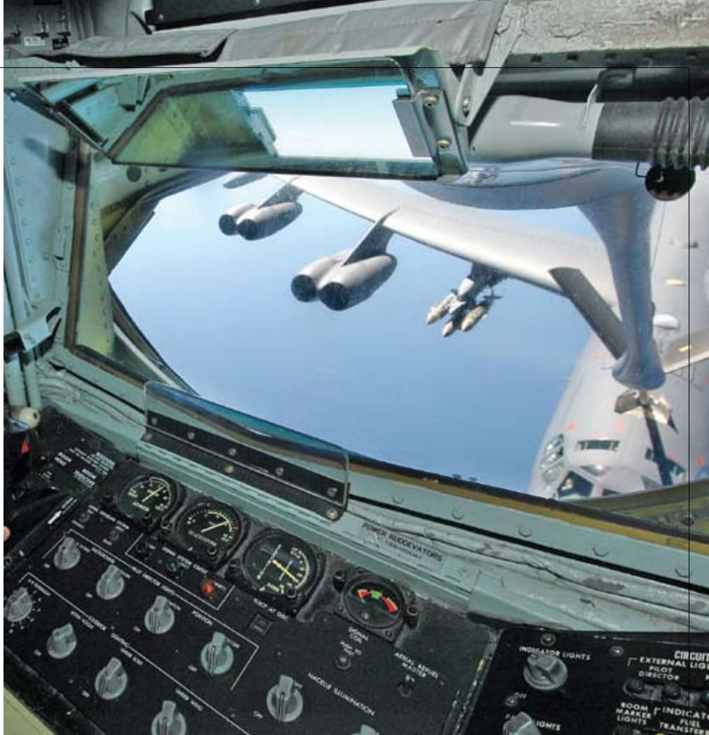
In a KC-135 Stratotanker, even the most routine fueling mission is an exciting adventure. April Widman ('04, EC/DL) lowers the tanker's boom into the waiting aircraft's fuel receptacle—a critical and precise maneuver she performs while cruising at 30,000 feet at about 500 miles per hour.
