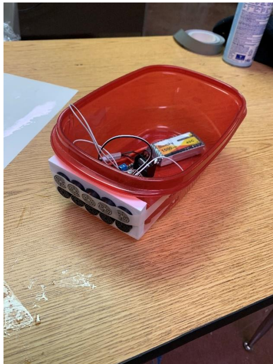
Fig. 2 Picture of Boat Configuration with One Row of Transducers Being Used (Bottom Row)
