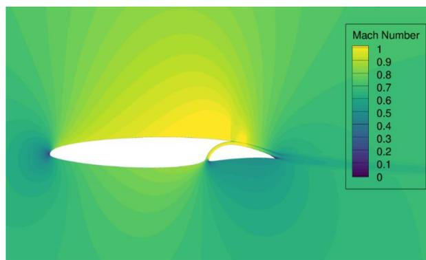
**Fig. 2 CFD image of S207, slotted, natural-laminar flow airfoil**
