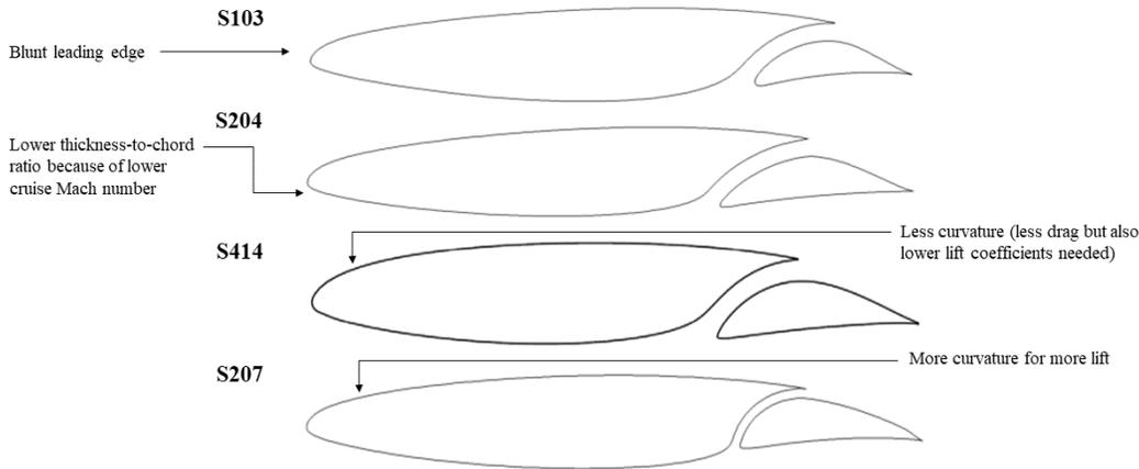
**Figure 9: Compilation of the SNLF airfoil images with design annotations [15]**
