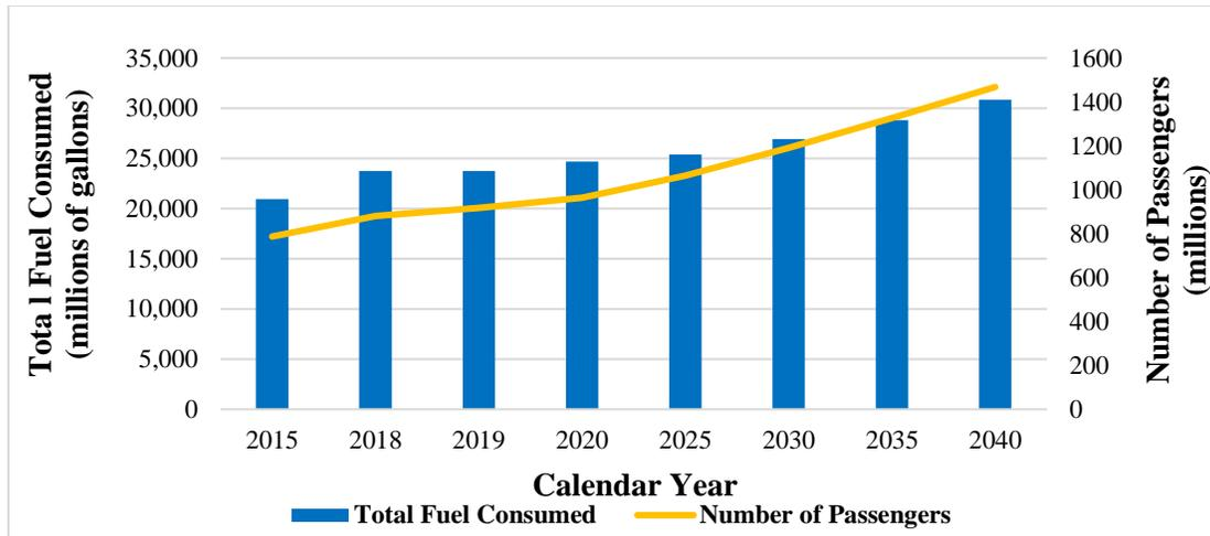
**Fig. 1 Total Domestic and International U.S. Passenger Traffic for U.S. Commercial Air Carriers; Historical and Projected Jet Fuel and Aviation Fuel Consumption by U.S. Civil Aircraft [1]**
