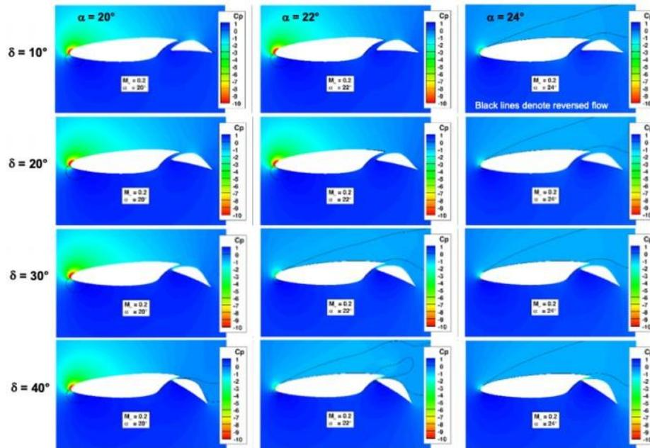
**Figure 10: Effect of Flap Deflection on the Flow Structure near Maximum Lift [22]**
