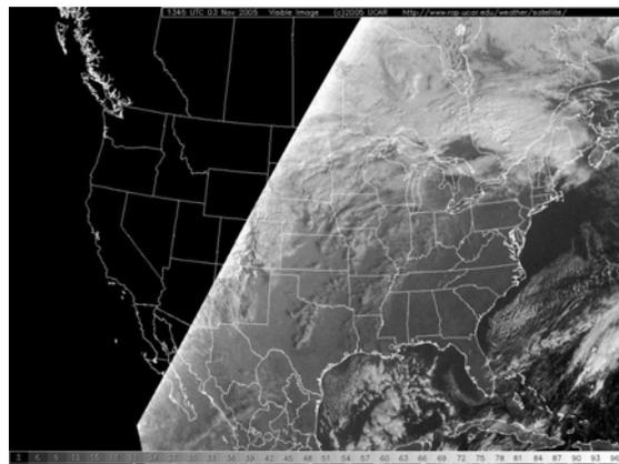
Figure 8. Visible GOES-east data at the same time as figure 7. The visible brightness has been divided by the cosine of the solar zenith angle.
