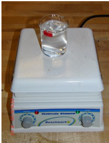
Figure 8: Stirring solution with hot plate and magnetic stirrer
