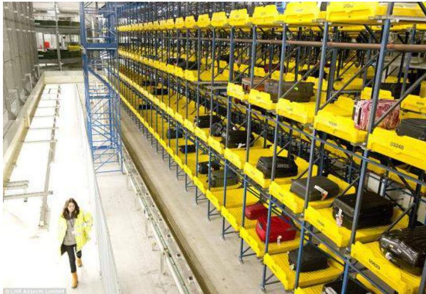
*Figure 4.* Heathrow Terminal 5 baggage handling system – Storage. Adapted from “Ever wondered what happens to your bag at an airport? Behind the scenes on the luggage conveyor belts of Heathrow Terminal 5”, by Duell, 2014. Retrieved from <http://www.dailymail.co.uk/news/>. Copyright 2014 by Duell.
