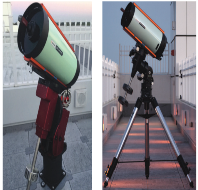
Software Bisque Paramount Losmandy with Gemini 2 Figure 1. Shows the telescope mounts that the OSCOM system currently supports.
