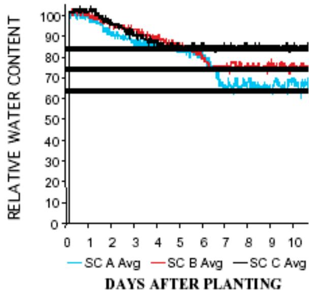
Figure 8. Set-point maintenance using moisture sensor feedback control.
