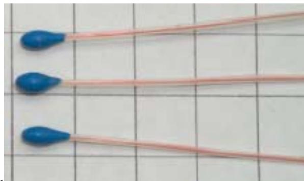
Figure 7. TMAS Heat Pulse Moisture Sensors. Grids = 1 cm.
