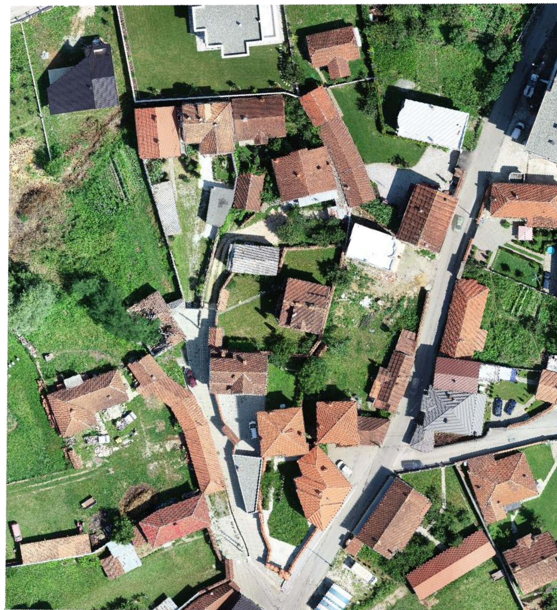
Figure 1: Pix4D model of a kulla and the surrounding area captured with the DJI Phantom 4 Pro
