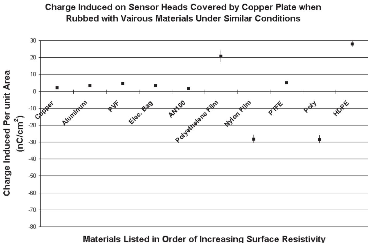
**Figure 2: Surface Resistivity and Triboelectric Charge Generation Comparison**
