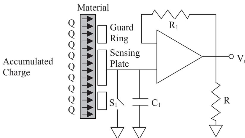
**Figure 1: Figure of triboelectric charge test device.**
