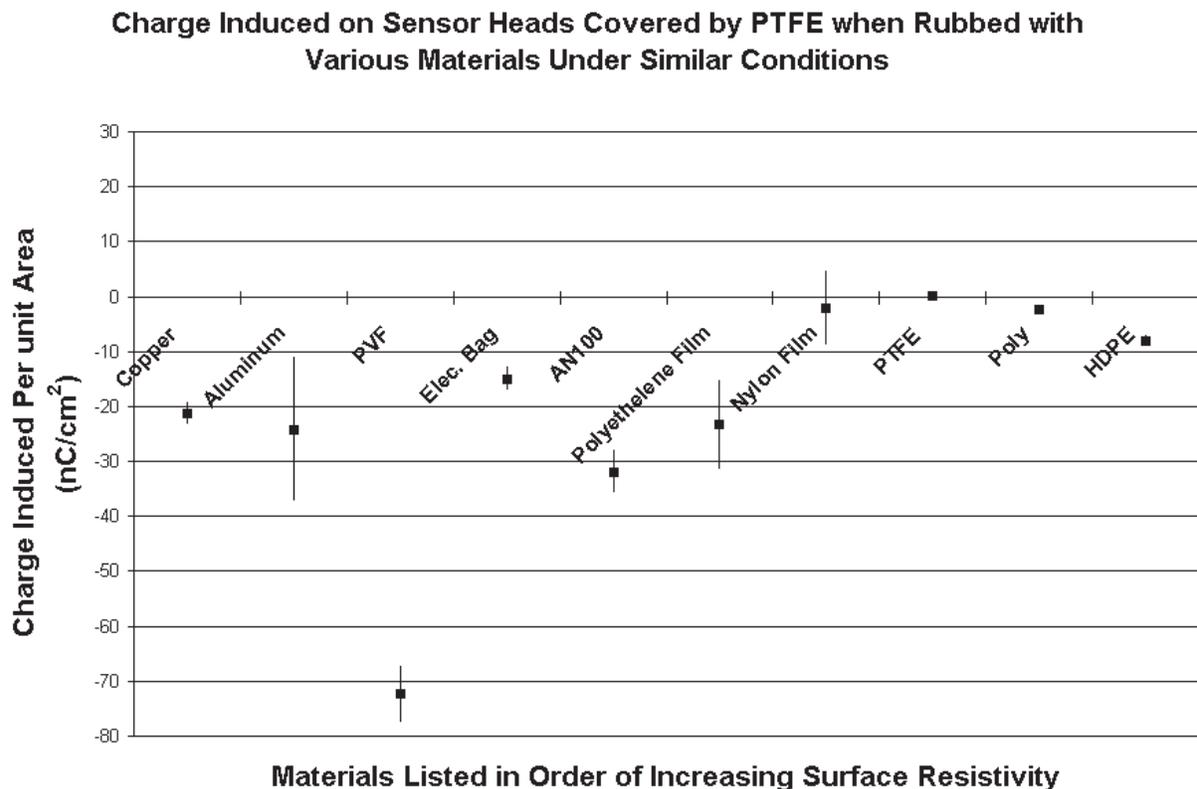
**Figure 3: Surface Resistivity and Triboelectric Charge Generation Comparison**
