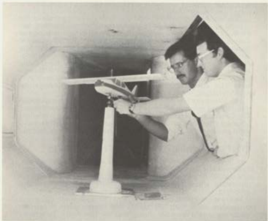
Graduate students prepare a model for wind tunnel testing.
