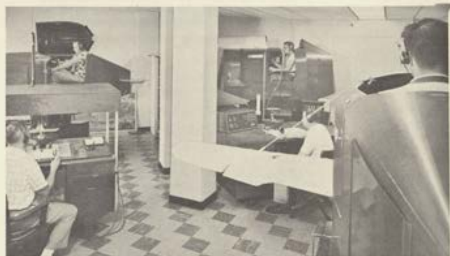
Link Trainers prepare for basic instrument procedures
