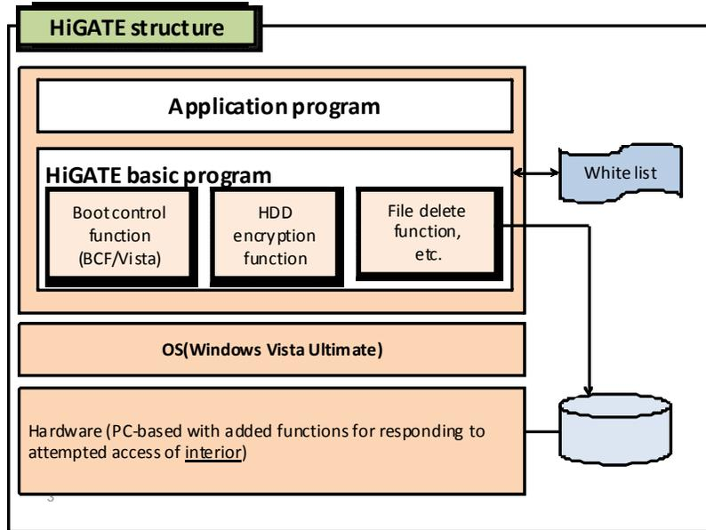
Figure 1. HiGATE Block Diagram
