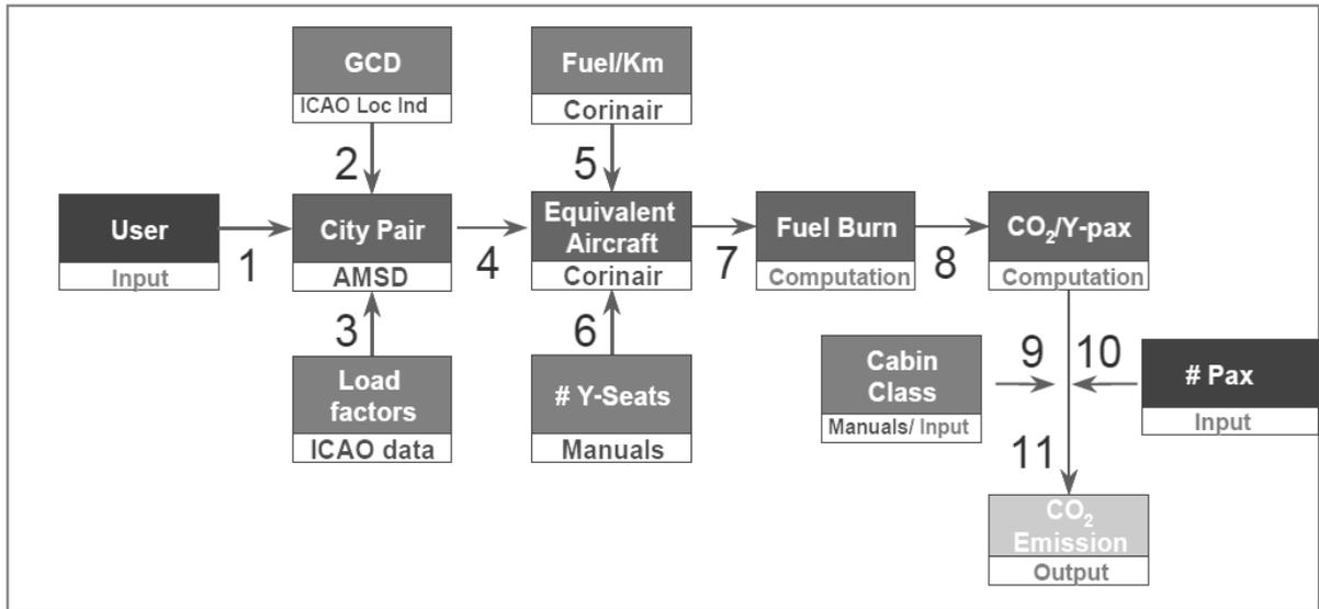
Figure 1. Flowchart of methodology used by ICAO /CORINAIR to determine the total emission of CO<sub>2</sub> produced by burning a ton of aviation fuel (ICAO, 2014)
