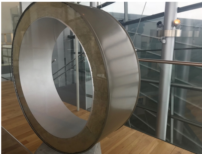
Photo 2: Cross-section of pipe used to transport geothermal-heated water throughout Reykjavik from Hellisheidavirkjun Power Plant. (Julianna Martorella, photograph, 14 Mar. 2018)
