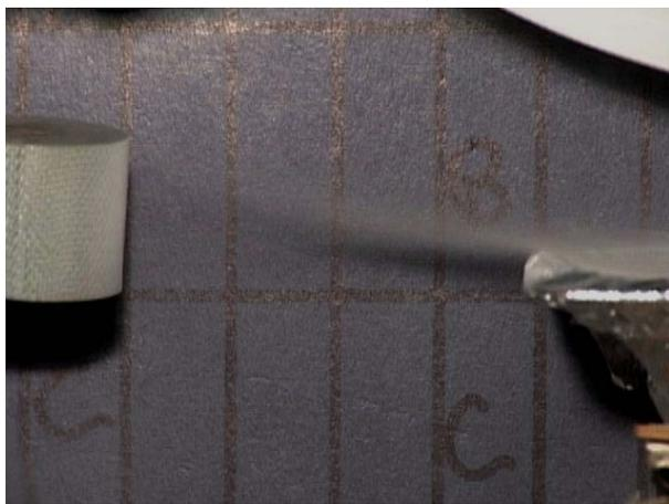
**Figure 3.** Dust particles being impelled towards the cylindrical electrometer. Photo taken through a viewport of a vacuum chamber being operated at 10 mb in CO<sub>2</sub> atmosphere.
