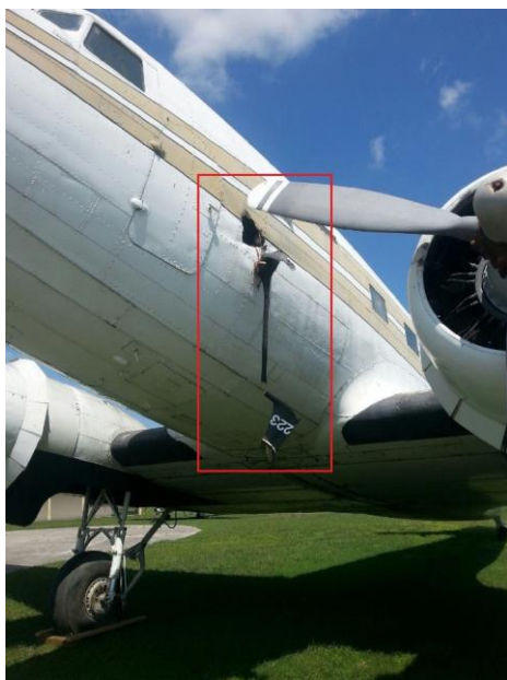
Figure 2. Damage caused by small prototype, fixed-wing UAS against a parked static aircraft. While this accident was inadvertent, the incurred damage demonstrates the kinetic destructive potential of UAS platforms (Used with permission).
