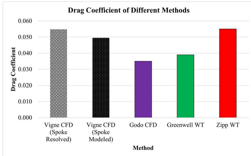
**Fig. 9 Drag coefficient comparison of HED Trispoke wheels at 30mph and 10 degrees AoA**
