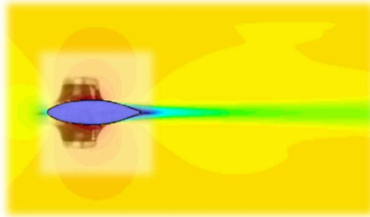
**Fig. 3 Spoke velocity profile at 100k Re and 0 degrees AoA with cross-section overlay**
