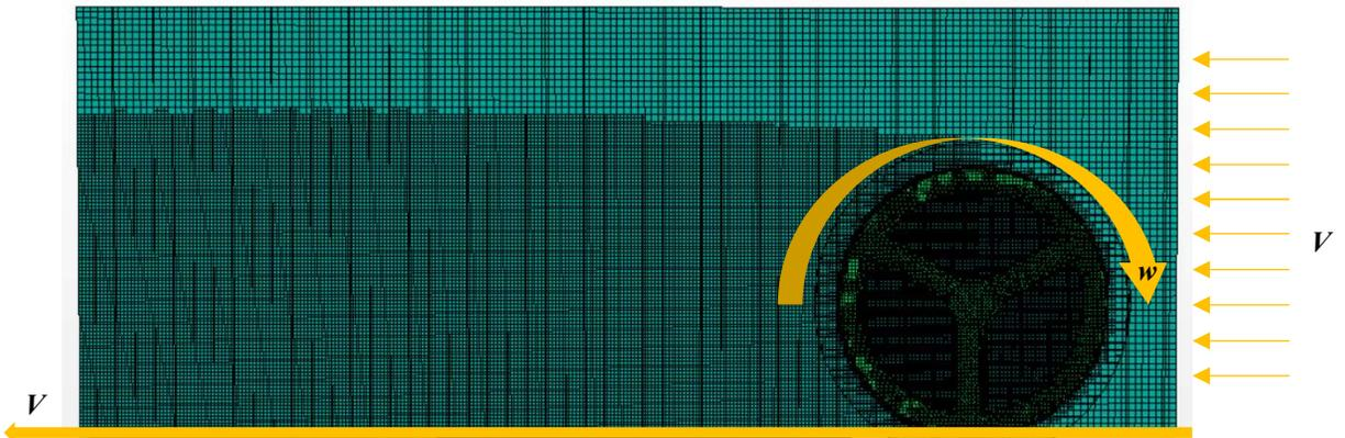
**Fig. 6 Mesh used in mesh refinement study**
