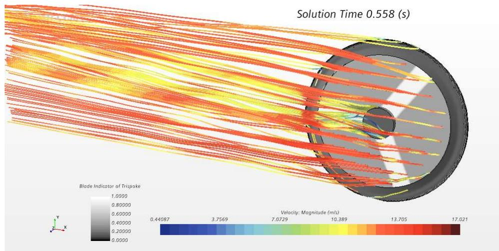
**Fig. 10 Blade Modeled streamlines with virtual disk shown as “Blade Indicator”**
