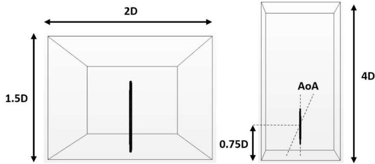
**Fig. 5 Computational domain front-view and top-view**
