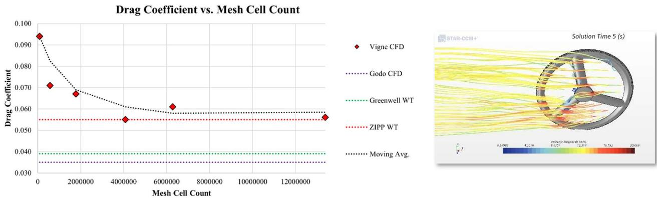
**Fig. 7 Mesh refinement study results and streamlines**
