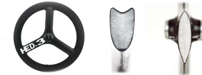
Fig. 1 HED TriSpoke side-view, rim cross-section, and spoke cross-section
