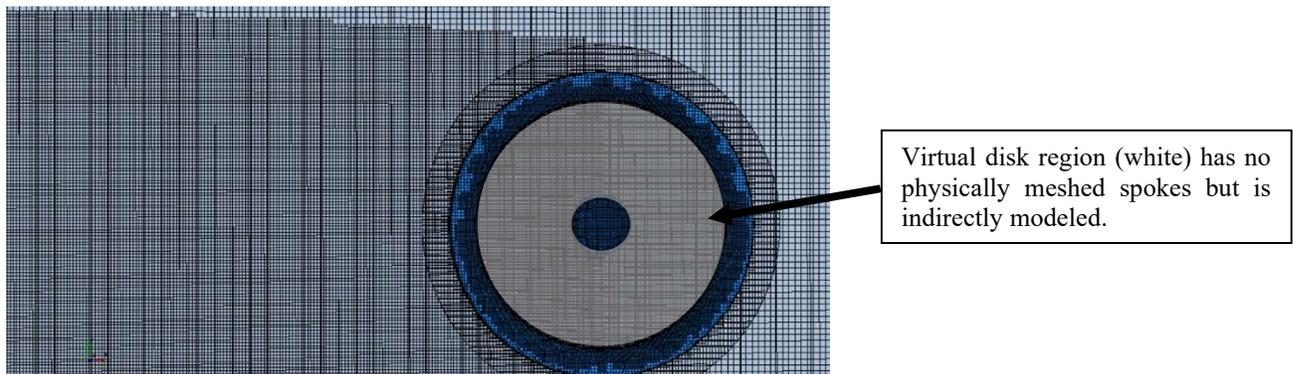
**Fig. 8 Spoke Modeled mesh domain**
