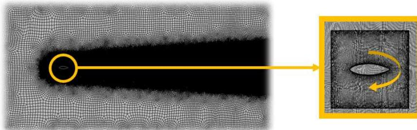
Fig. 2 Spoke Analysis 2D rotating overset mesh
