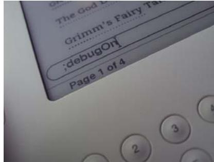
**Figure 3 - The “;debugOn” command being issued**
