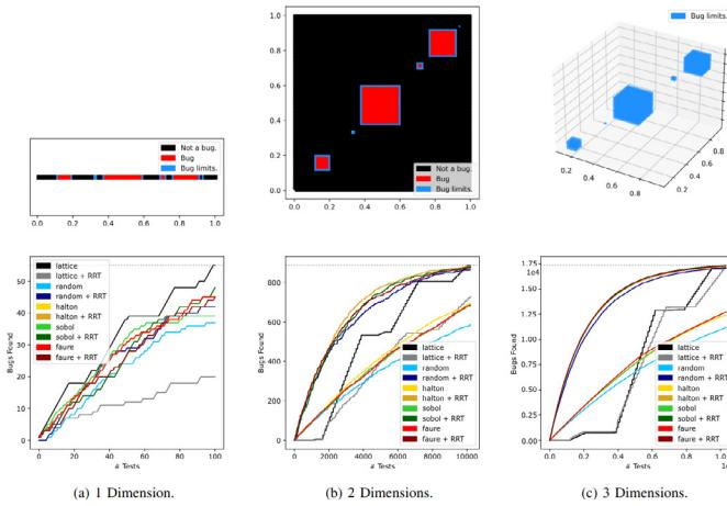
*Figure 1:* Comparison of approaches from one to three dimensions. (Top) Distribution of bugs. (Bottom) Total unique bugs found as tests are run.
