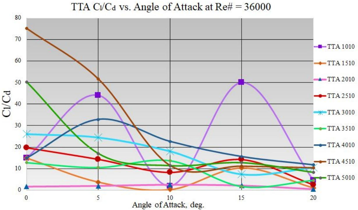
**Fig. 6 Graph of each airfoil tested at a single  $Re\#$**
