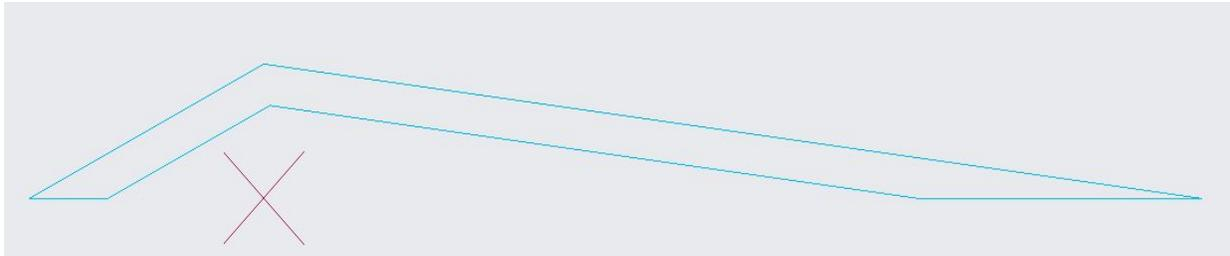
**Fig. 1 An engineering drawing of the TTA-2010 airfoil. Notice, the cross mark denotes the location of the max camber point.**
