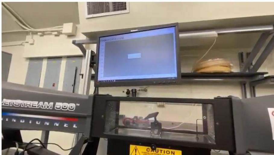
**Fig. 5 A TTA in the Jetstream 500 wind tunnel.**
