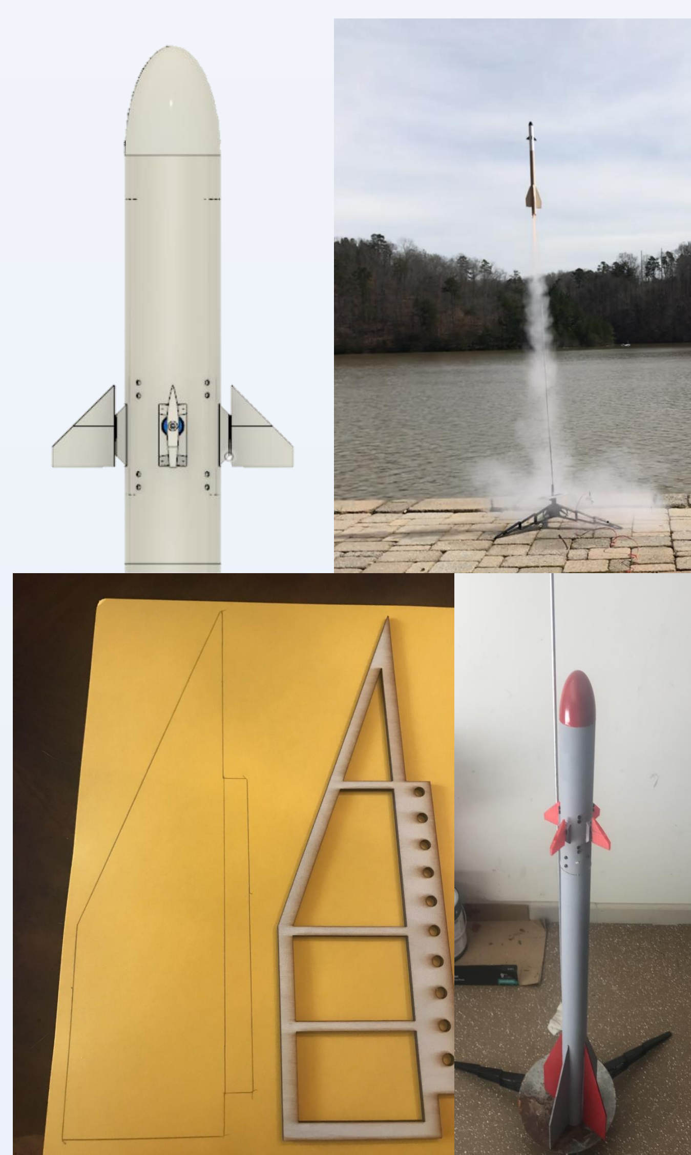
Top Left: Model of Freefall's upper section. Top Right: Launch of "Nosedive" scale model of Freefall. Bottom Left: Lattice Fin shortly before assembly. Bottom Right: Completed Freefall rocket with stabilization system installed.
