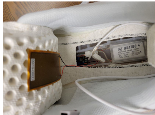
Figure 9: Shoe Prototype with Circuit Placed Inside
