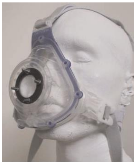
Fig. 2 Collection Mask used in Viral Aerosol Study [2]
