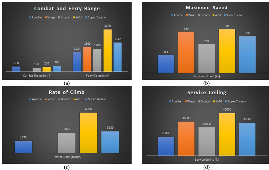
Figure 4 Comparison of Aircraft Performance: (a) Combat and Ferry Range, (b) Maximum Speed, (c) Rate of Climb, (d) Service Ceiling.
