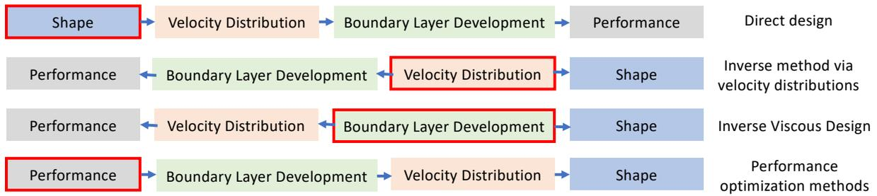
Figure 4: Comparison of approaches to Airfoil Design adapted from literature<sup>13</sup> and presented in flowchart form for one design cycle.
