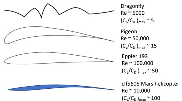
Figure 3: Typical cross-section shapes of low Re airfoil and efficiency from literature<sup>5</sup> adapted to include comparison with the Mars helicopter airfoil clf5605<sup>8, 18</sup>
