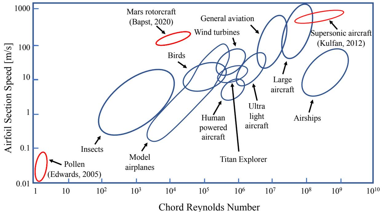
Figure 1: Section speed vs Reynolds number plot categorizing the various lifting surfaces according to type of operation adapted from literature<sup>5,6</sup> with added categories in red<sup>2</sup> including values for more recent aerial applications for planetary exploration such as the Mars helicopter.<sup>7,8</sup>
