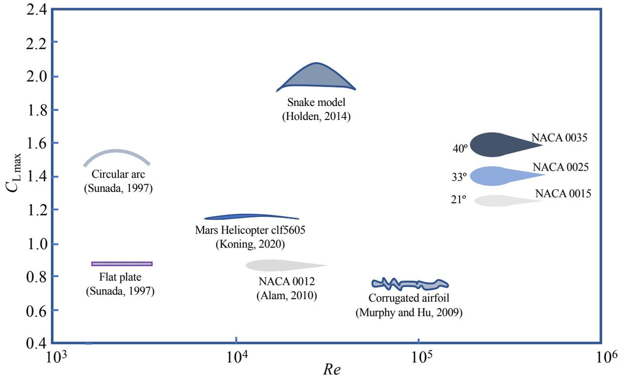
Figure 2: Maximum Coefficient of Lift vs Reynolds number plot with the stall angle listed categorizing some examples of lifting surfaces in the low Re region. This is adapted from literature<sup>16</sup> with the addition of data from airfoil geometries for more recent aerial applications for planetary exploration such as the Mars helicopter<sup>7, 8, 18</sup>
