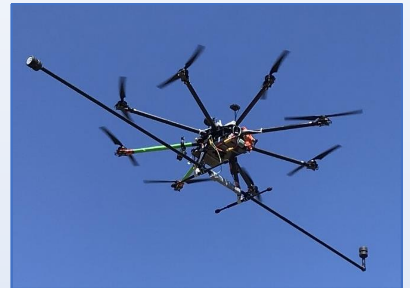
Figure 1: Tarot-T18 used for flying the Vaisala AQT 4000 sensor.
