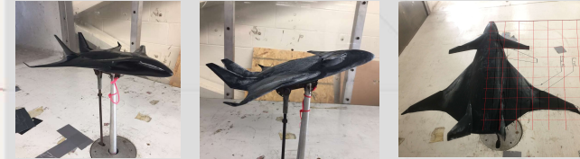
Figure 5. Model on test-stand (superimposed grid provides positional information for clay flow visualization)
