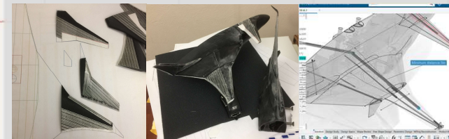
Figure 4. Model construction showing trailing edge build up and internal reinforcements (Right)
