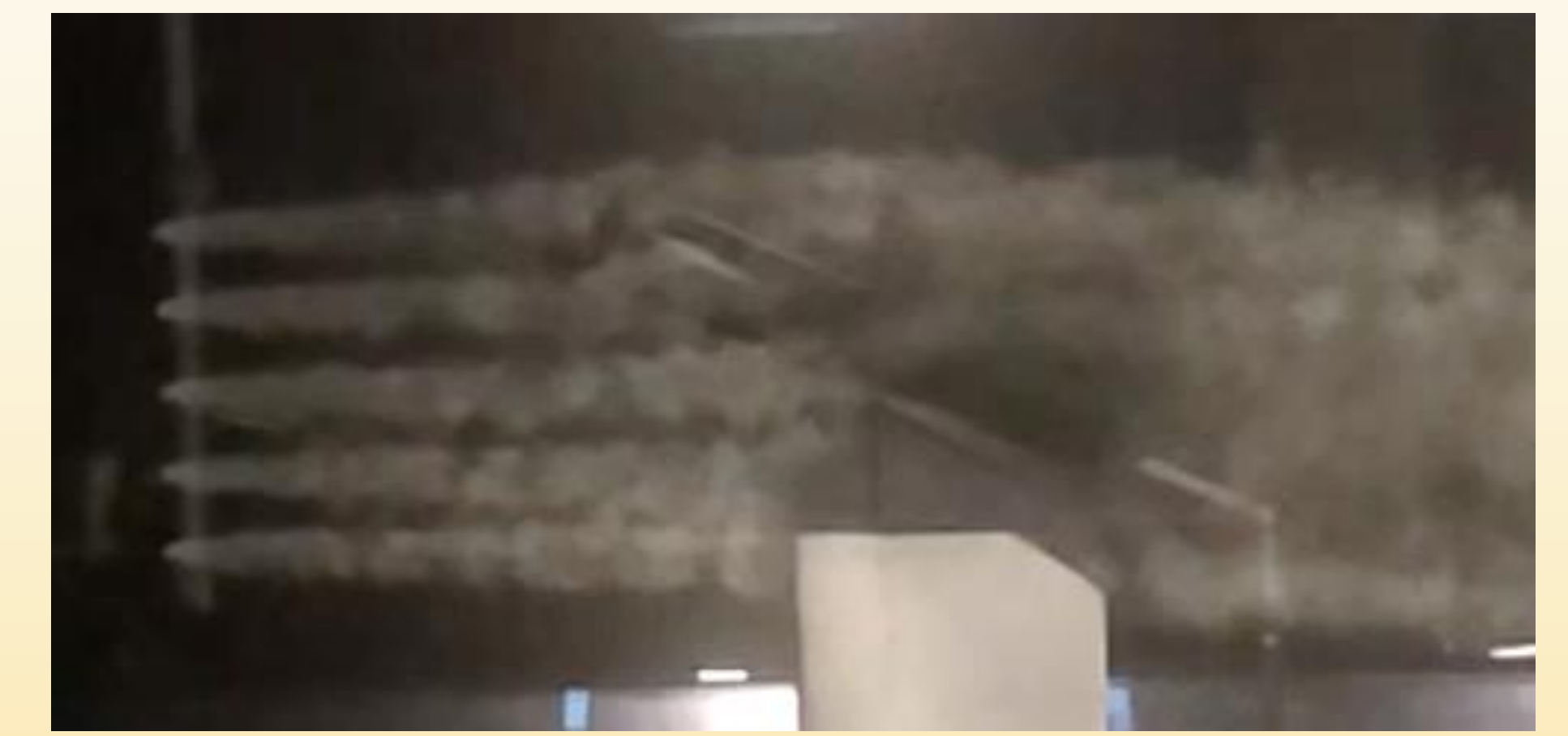
Figure 7. Sheet of smoke created at 10ft/s.
