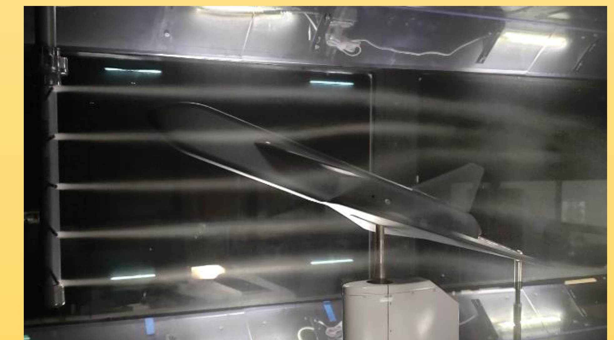
Figure 8. Flow from the front canard wing can be seen effecting the streaklines in the center of the image.
