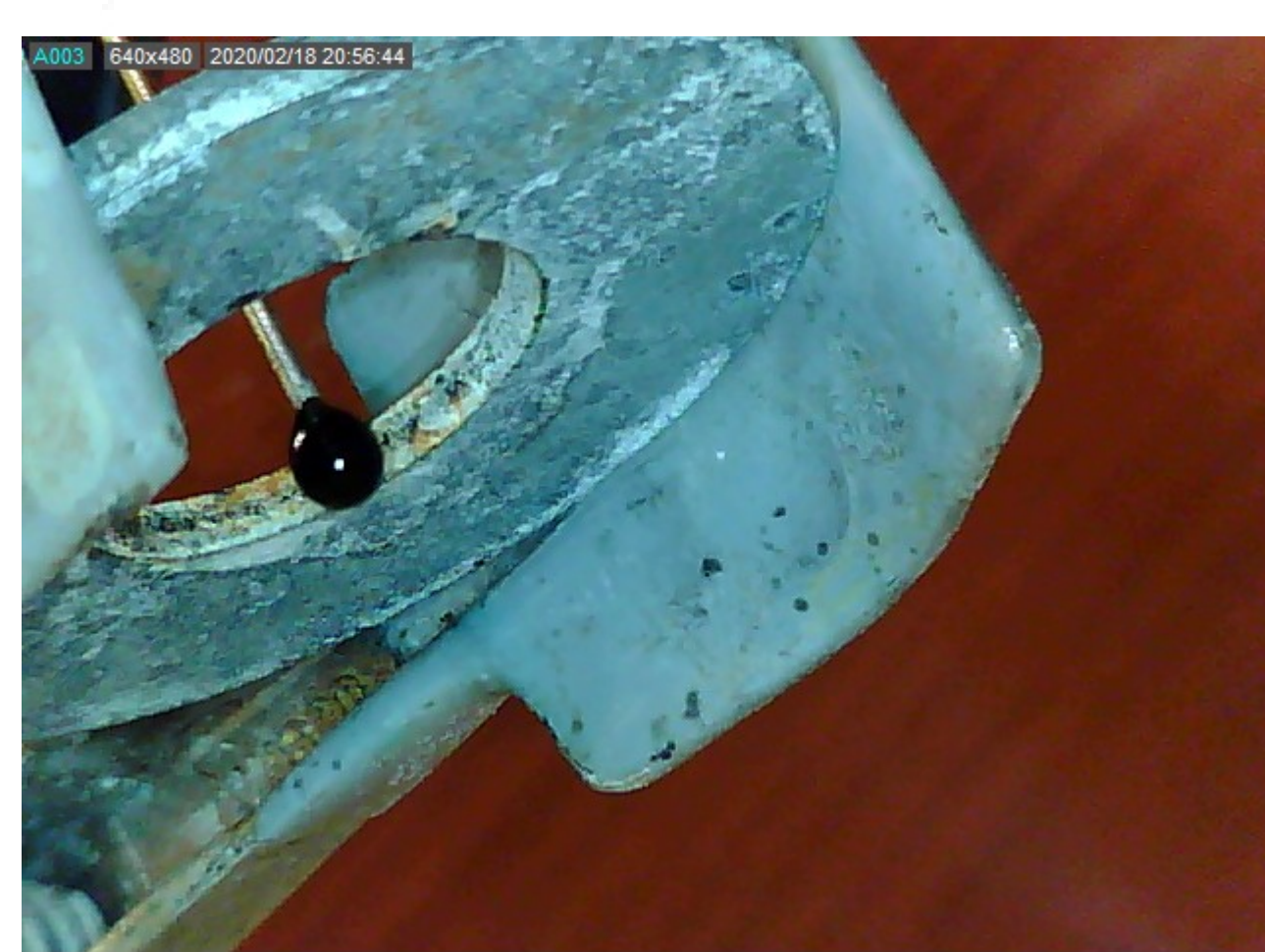
Fig. 2, 3: Formation of Taylor cone as the electromagnetic attraction overcomes the surface tension of the CNT solution.
