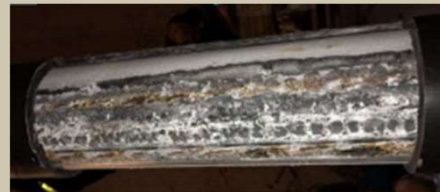
Shows the top of a tendon found in the Ringling bridge with deficient grout and strand corrosion
