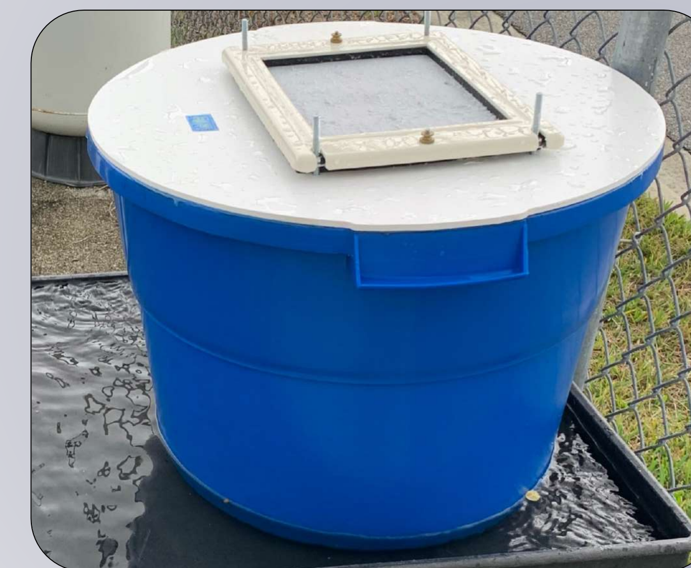
Figure 4: Passive sampling setup.
