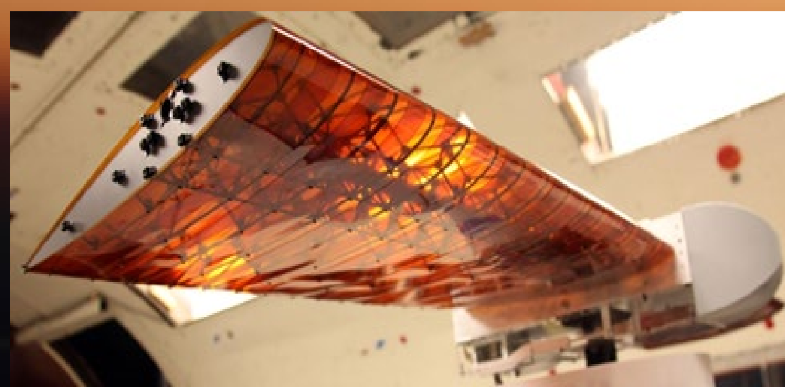
Figure 1: Morphing wing with active cellular structure (2017 Jenett, B., Calisch, S., Cellucci, D., Cramer, N., Gershenfeld, N., Swei, S., & Cheung, C. K. (2017). Digital Morphing Wing: Active Wing Shaping Concept Using Composite Lattice-Based Cellular Structures. Soft Robotics , 4(1), 33-48.
