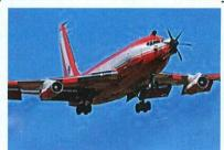
either to a museum or a scrapyard. The engine maker has replaced it with a Boeing 747 SP. The 720 was a stubby version of the 707 and was designed for shorter fields. Paradoxically, even though it could get into tighter places, it was faster than the 707. There were 64 720s built along with 88 720B models with turbofan engines.
