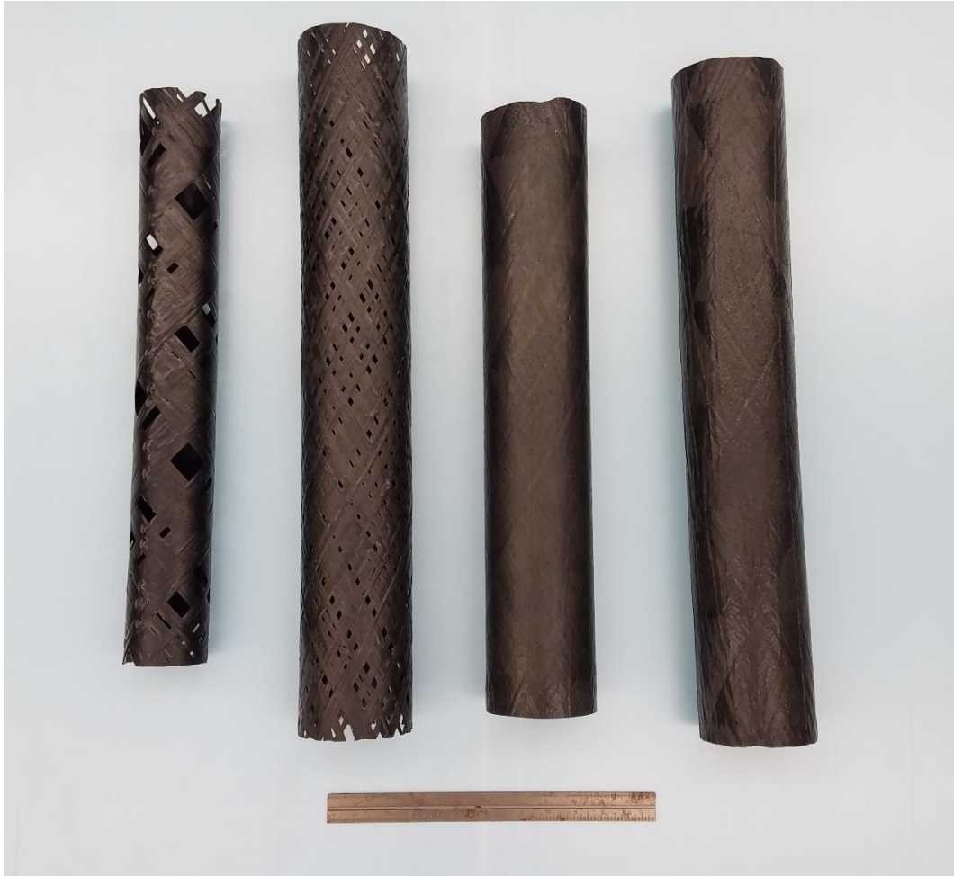
Figure 6: Tubes are arranged in order of iteration. From left to right: Iteration 1, Iteration 2, Iteration 3, Iteration 4. Iteration 4 was used as the airframe in the flight test. A 12-inch ruler is positioned along the bottom for scale.
