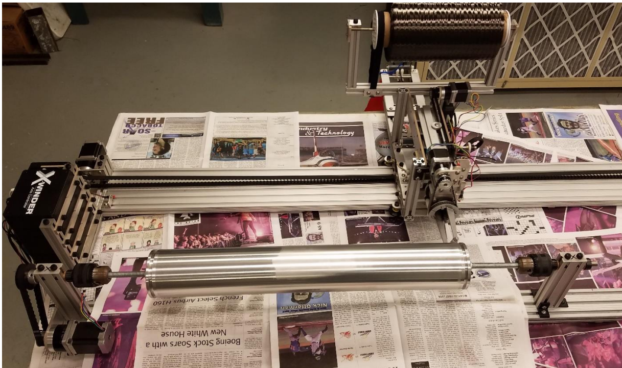
Figure 5: The X-Winder filament winder set up for manufacturing.
