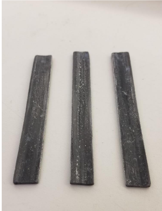
Figure 4: Finished product of carbon fiber coupons cut to length. These were never tested due to poor quality of manufacturing.
