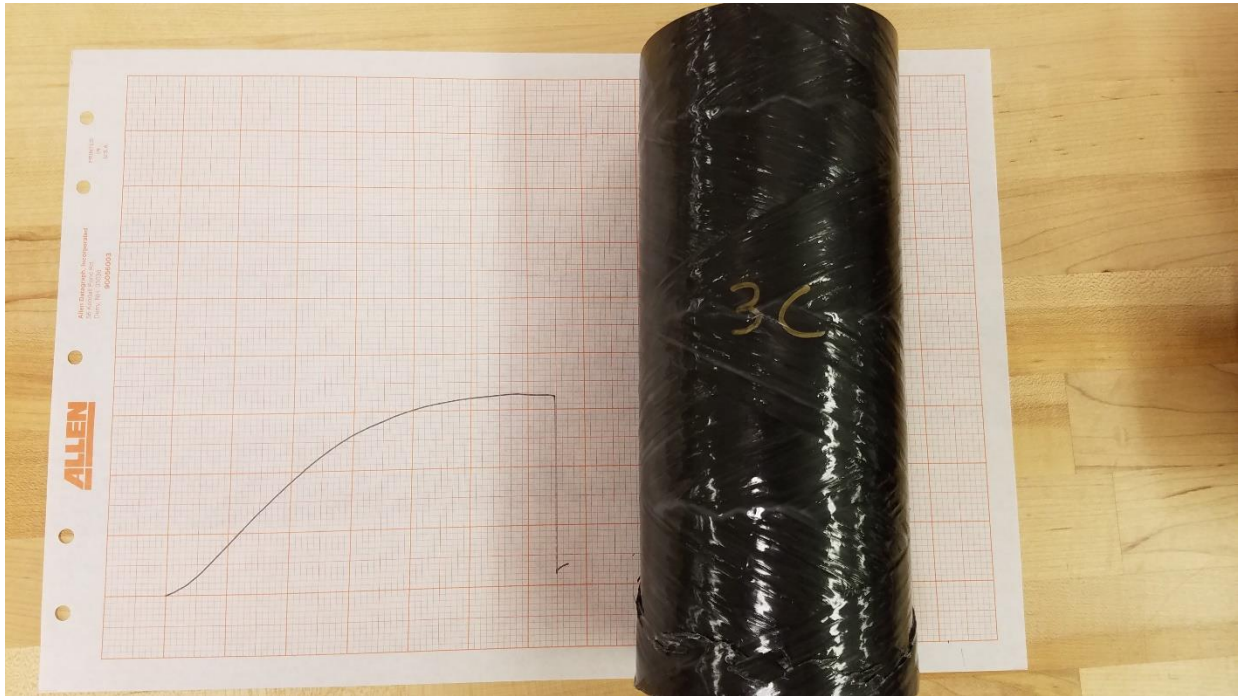
Figure 10: Tube 3C after it had been through its compression test with its Force VS Displacement curve
