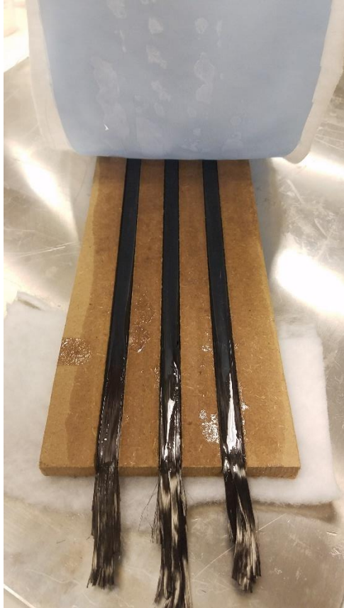
Figure 3: A picture of the carbon fiber coupons in manufacturing prior to vacuum bagging.
