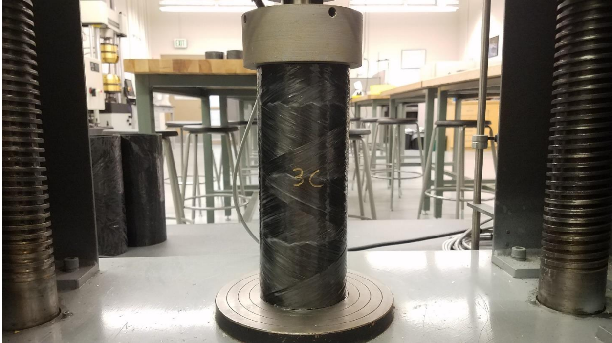
Figure 13: Tube 3C in its test configuration in the Tinius Olsen LoCap Testing Machine just prior to test.
