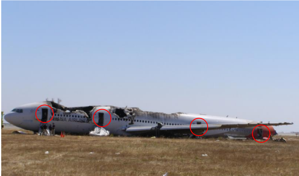
Image 17. Left side of Flight 214 from the 9 o'clock position depicting doors 1L, 2L, 3L, 4L.
