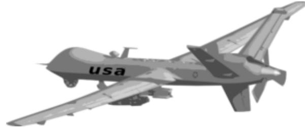
**An UAS is not merely an aircraft but in systems engineering terms, a “system of systems” consisting of the aircraft, the ground station, the GPS satellite constellation, the communication infrastructure (L-Band, C-Band), the launch & recovery infrastructure, the personnel, etc.**
