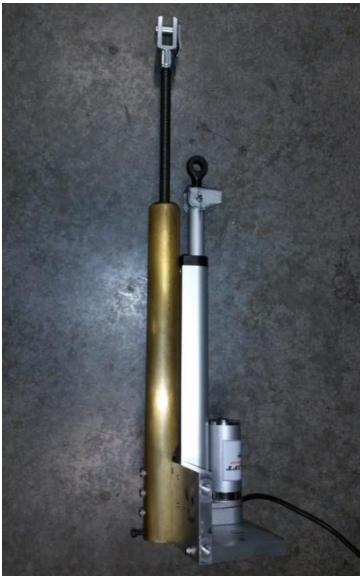
Figure 7. The balance bar with brass test article attachment rod, and linear actuator with mounting platform.
