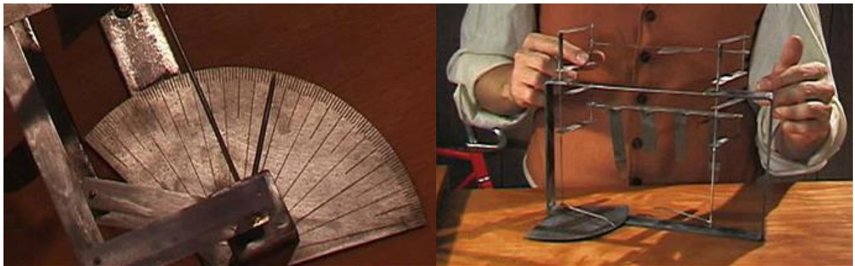
Figure 2 . The balances used in the Wright brother’s first wind tunnel
