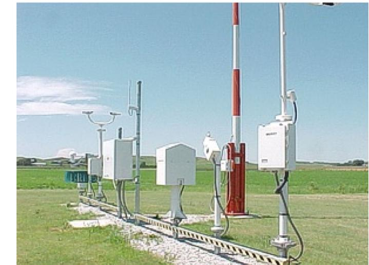
**Figure 2.** Above is a photograph of ASOS equipment recording weather data provided by NWS and NOAA. This equipment is located in the Raleigh area and runs non-stop, updating weather observations every minute 24 hours a day. The ASOS network has more than double the number of full-time service surface weather observing locations in the NWS Raleigh Country Warning Area.
