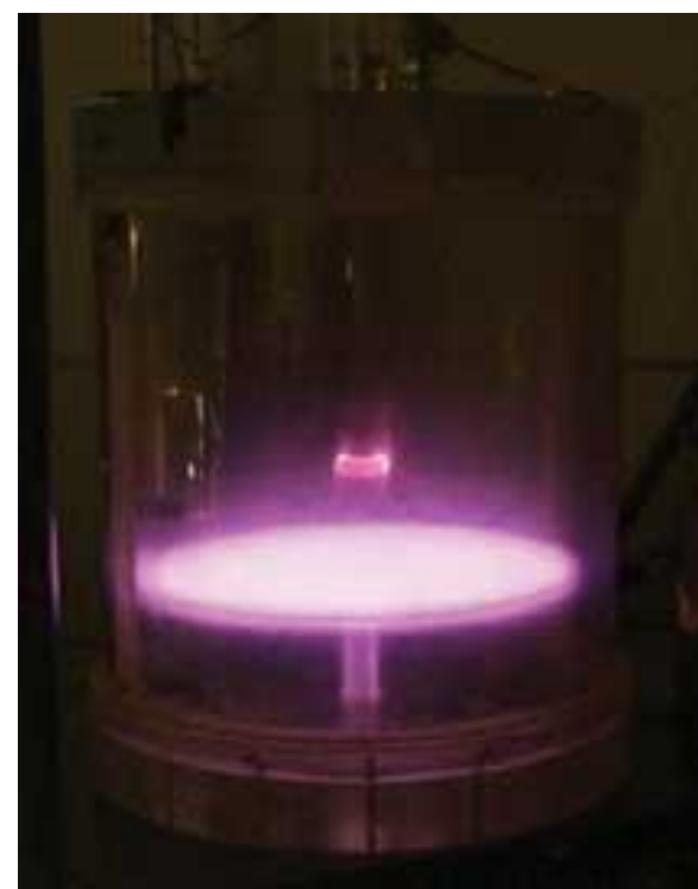
Figure 1: Dusty Plasma Experiment chamber located at the Naval Research
