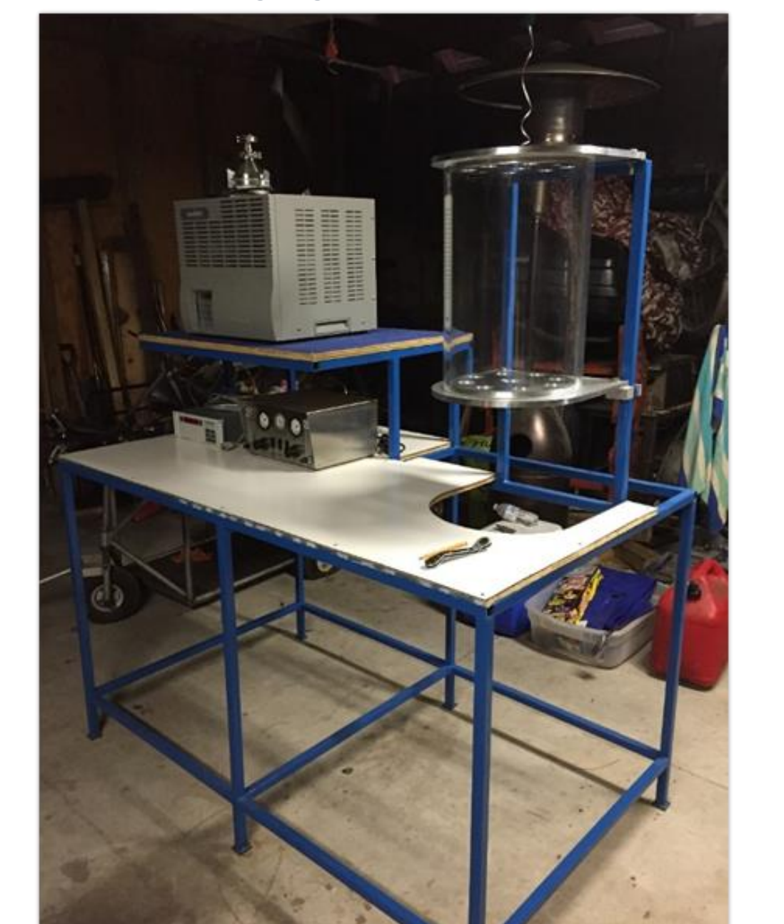
Figure 5: Progress photo of the tubing, the end flanges, the turbomolecular pump, the gas flow controller, and the active digital gauge controller.
