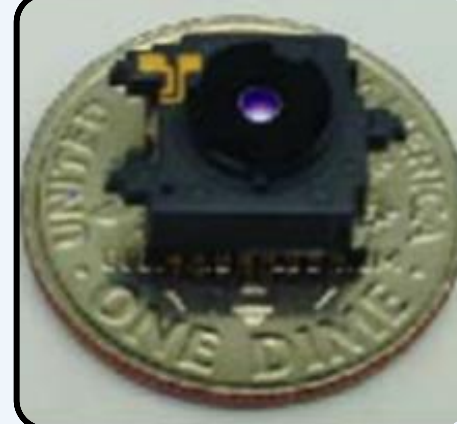
FLIR Lepton with a dime for size comparison.
